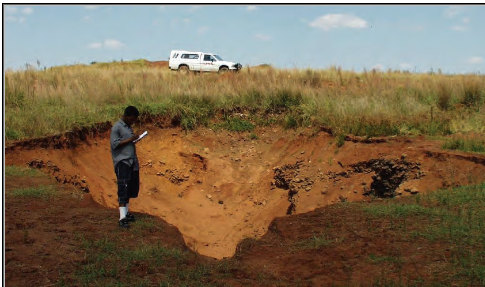
Figure 10.4: One of the sinkholes in the dry streambed of the Tweelopiespruit West immediately downstream from Tarlton. These sinkholes were formed due to the increased flow in the stream and also due to the removal of the peat beds in this stream (run-off attenuation properties of peat lands and associated reed beds), allowing storm water to flow further downstream before recharging into the dolomitic aquifer (photo: W.G. Krige 31/03/2002).
